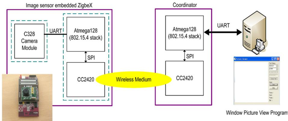
Fig. 4. Connection layout between the camera device and coordinator.
