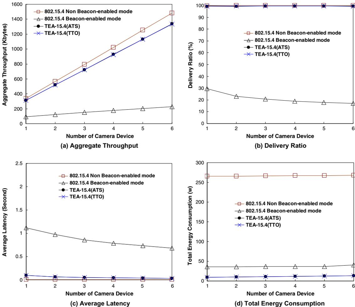
Fig. 12. Results for various numbers of image sensors with SO = 5, BO = 8 and nodes = 50.
