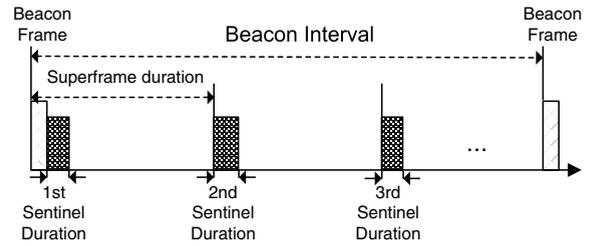
Fig. 8. Performing sentinel durations in a beacon interval.
