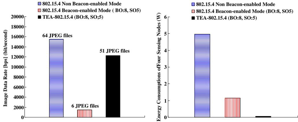
**Fig. 10.** Experimental results in the TEA-15.4 and 802.15.4 Non-Beacon-enabled/Beacon-enabled modes: Image data rate, Number of received JPEG files, and Energy consumption.
