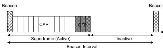
Fig. 2. Superframe structure in the IEEE 802.15.4 Beacon-enabled mode [7].
