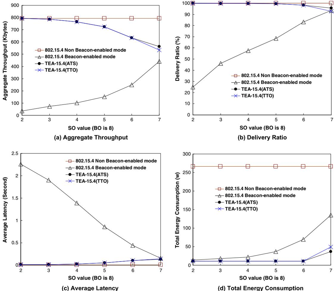
Fig. 13. Results for various SO values with BO = 8, scalar sensors = 50, and image sensors = 3.
