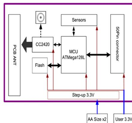
Fig. 3. The real sensor platform: ZigbeX.
