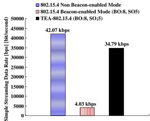
**Fig. 11.** Experimental results in the proposed TEA-15.4 scheme and the IEEE 802.15.4 Non-Beacon-enabled/Beacon-enabled modes: Streaming data rate (bps).
