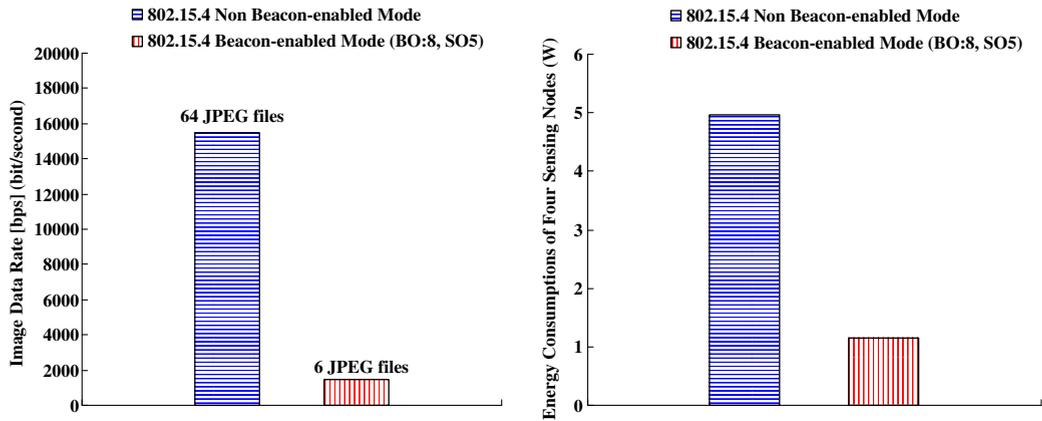
Fig. 6. Experimental results in 802.15.4 Non-Beacon-enabled and Beacon-enabled modes: Image data rate, Number of received JPEG files, and Energy consumption.
