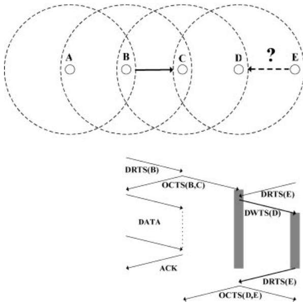
Fig. 10. Example of using DWTS frames.
