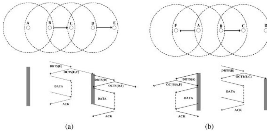
Fig. 2. Examples of using a directional MAC scheme 1.
