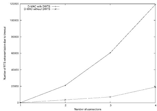
Fig. 12. Result for number of unnecessary RTS retransmission by varying the number of adjacent connection(s).
