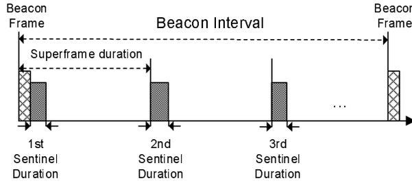
**Fig. 1.** Performing sentinel durations in a beacon interval
