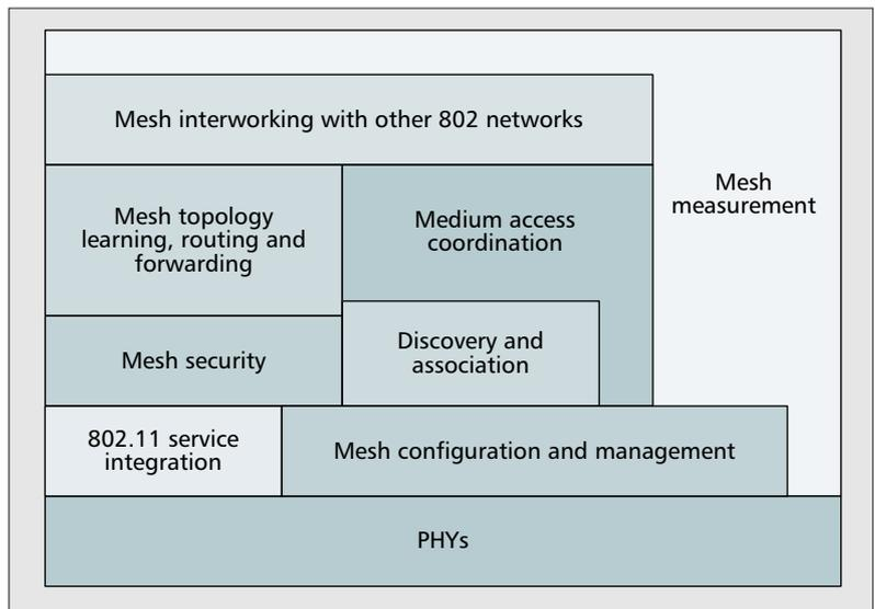
Figure 3. Architecture for the 802.11s MCF sublayer.
