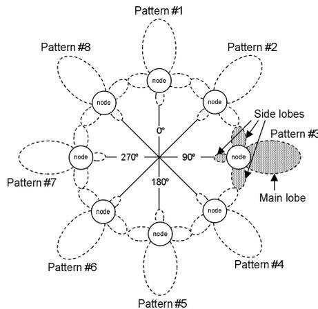
Fig. 2. The simplified pattern of directional antenna
