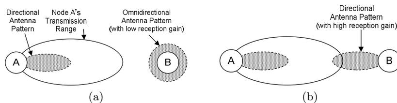
**Fig. 1.** An example showing the effect of the receiver's different antenna pattern on the success of communication
