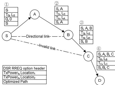
Fig. 4. Flooding of RREQ with DAPOS
