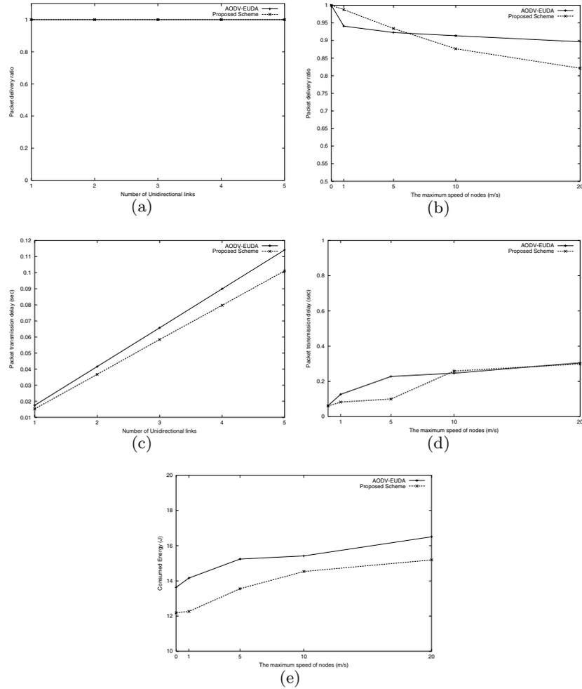
**Fig. 3.** Results on (a) Packet delivery ratio in static model (b) Packet delivery ratio in mobility model (c) Delay in static model (d) Delay in mobility model (e) Energy consumption
