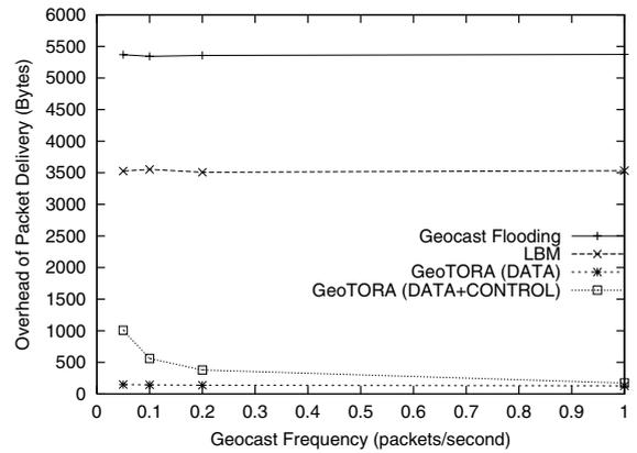
Fig. 13. Average number of bytes versus geocast frequency.
