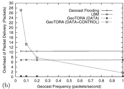
Fig. 12. Comparison of GeoTORA to geocast flooding and LBM protocols with a variation of geocast frequency (for 30 nodes, and pause time 10 s): (a) delivery accuracy versus moving speed, (b) average number of packets received by a node per geocast versus geocast frequency.
