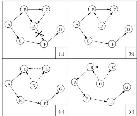
Fig. 1. An example of link reversal algorithm in route maintenance phase of TORA: Route maintenance is required due to failure of the link between nodes D and F.
