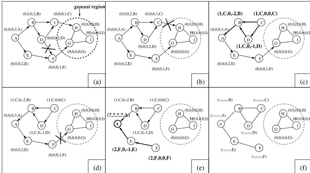
Fig. 6. Geocast route maintenance in GeoTORA: Three different scenarios of link failure.
