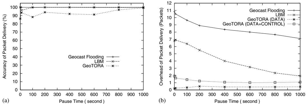
Fig. 8. Comparison of GeoTORA to geocast flooding and LBM protocols with a variation of *pause time* (for 30 nodes, and maximum speed 5.0 units/s): (a) delivery accuracy versus pause time, (b) average number of packets received by a node per geocast versus pause time.
