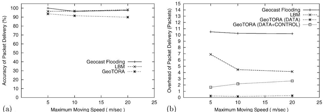
Fig. 10. Comparison of GeoTORA to geocast flooding and LBM protocols with a variation of *speed* (for 30 nodes, and pause time 10 s): (a) delivery accuracy versus moving speed, (b) average number of packets received by a node per geocast versus moving speed.
