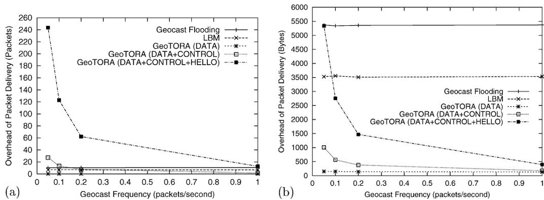
Fig. 16. Overhead comparison of GeoTORA to geocast flooding and LBM protocols with a variation of geocast frequency (for 30 nodes, and pause time 10 s): (a) overhead of geocast delivery (packets), (b) overhead of geocast delivery (bytes).
