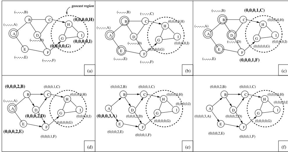
Fig. 5. Geocast route creation in GeoTORA.
