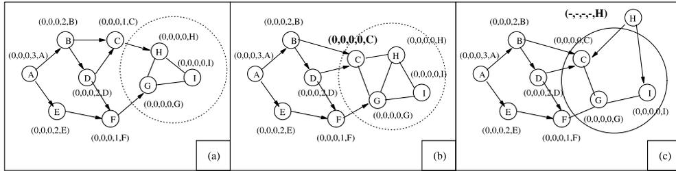
Fig. 7. Route maintenance in GeoTORA for handling dynamic change of geocast group.
