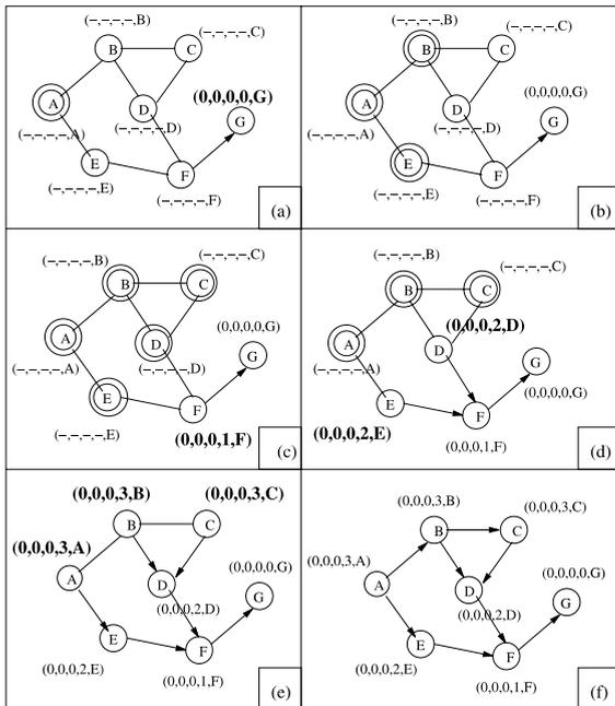
Fig. 4. Route creation phase in TORA: In the figure, a circle around a node indicates that the route-required flag is set. Arrows on each wireless link points from the higher height node to the lower height node. The height is depicted as a five-tuple, as explained in the context.
