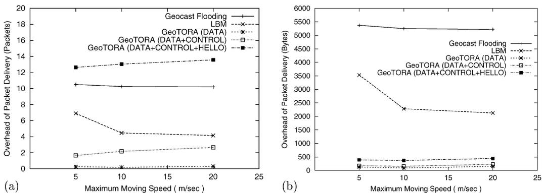
Fig. 15. Overhead comparison of GeoTORA to geocast flooding and LBM protocols with a variation of maximum speed (for 30 nodes, and pause time 10 s): (a) overhead of geocast delivery (packets), (b) overhead of geocast delivery (bytes).
