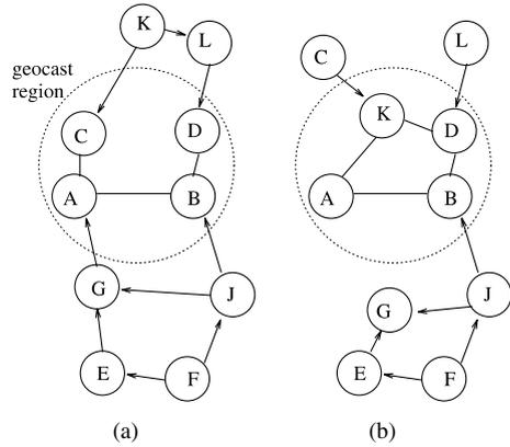
Fig. 3. Geocasting using GeoTORA.
