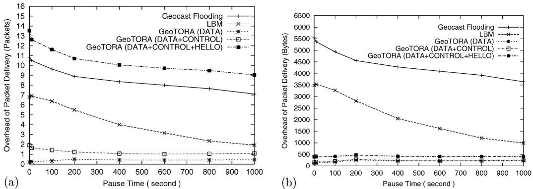
Fig. 14. Overhead comparison of GeoTORA to geocast flooding and LBM protocols with a variation of *pause time* (for 30 nodes, and maximum speed 5.0 units/s): (a) overhead of geocast delivery (packets), (b) overhead of geocast delivery (bytes).
