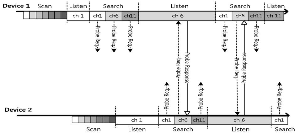
Figure 1. Device Discovery Process in Wi-Fi Direct[2]
