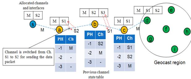
Fig. 2: MIMC-based Forwarding Scheme
