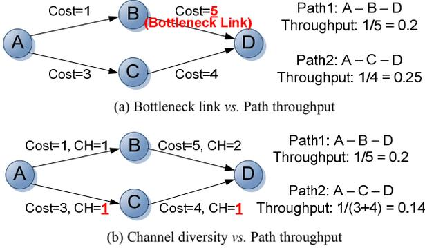
Figure 3. Two elements that affect path throughput
