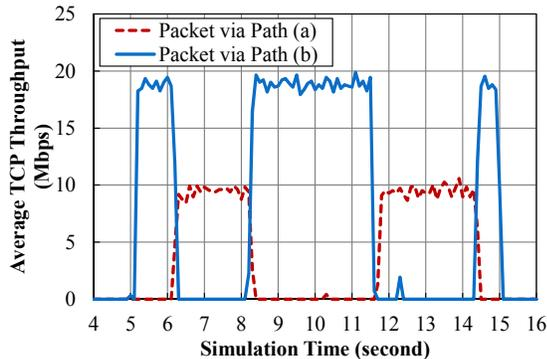
Figure 2. Path instability of the HWMP
