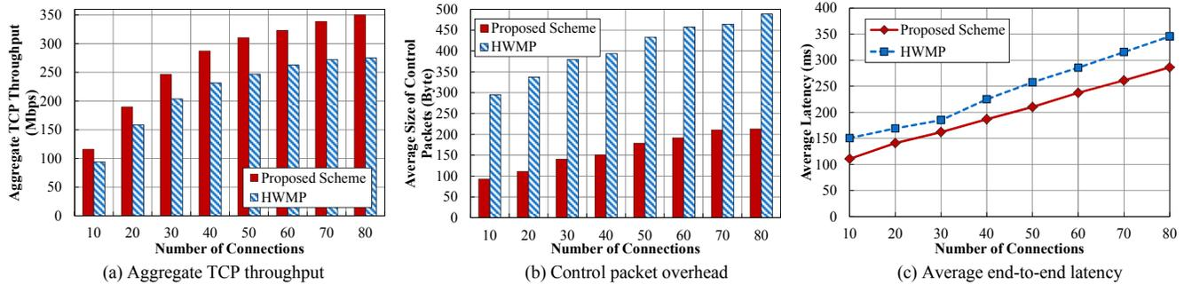
Figure 5. TCP performance results varying the traffic load
