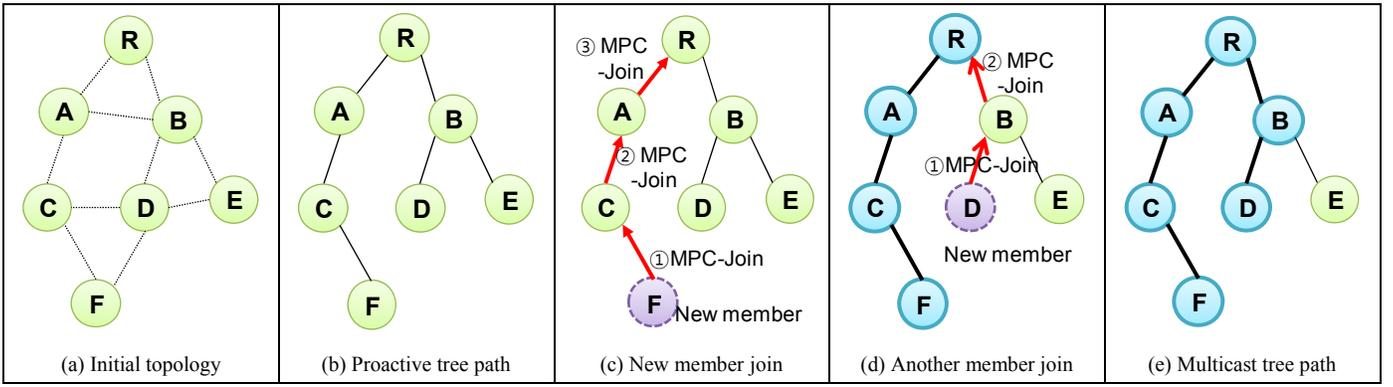
Fig. 2. An example of multicast tree construction in the proposed Scheme 1
