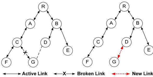
Figure 2. Examples of the first phase – Alternative parent node
