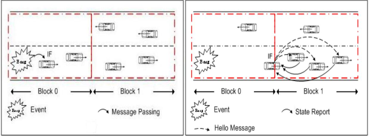
Fig. 1. (a) Mobile node sensing one urgent event becomes the initial ferry. (b) Ferry broadcasts hello messages upon entering into a new block.
