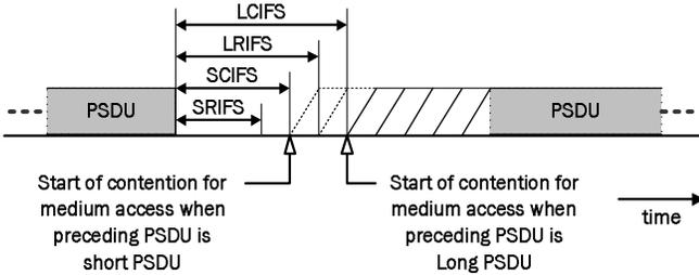
Fig. 1. Four different types of Inter Frame Space
