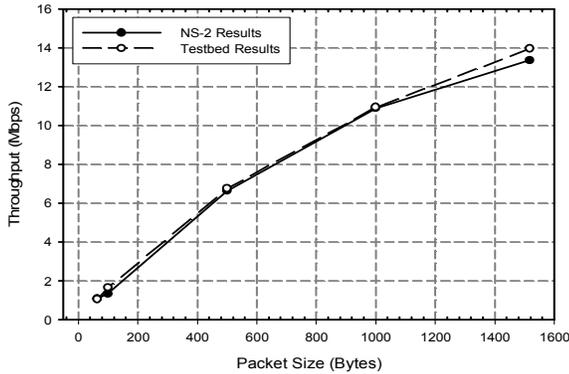
Fig. 10. Comparison of Throughput Depending on the Packet Size (Uni-directional transmission)
