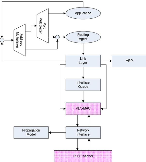
Fig. 4. Architecture of each PLC-Node in NS-2
