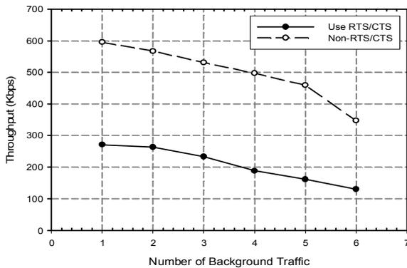
Fig. 14. Throughput of the Main Traffic According to the Number of Background Traffic
