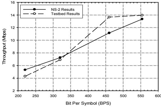
Fig. 9. Comparison of Throughput Depending on the BPS (Uni-directional transmission)
