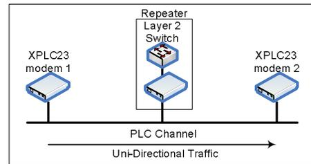
Fig. 12. Testbed Topology
