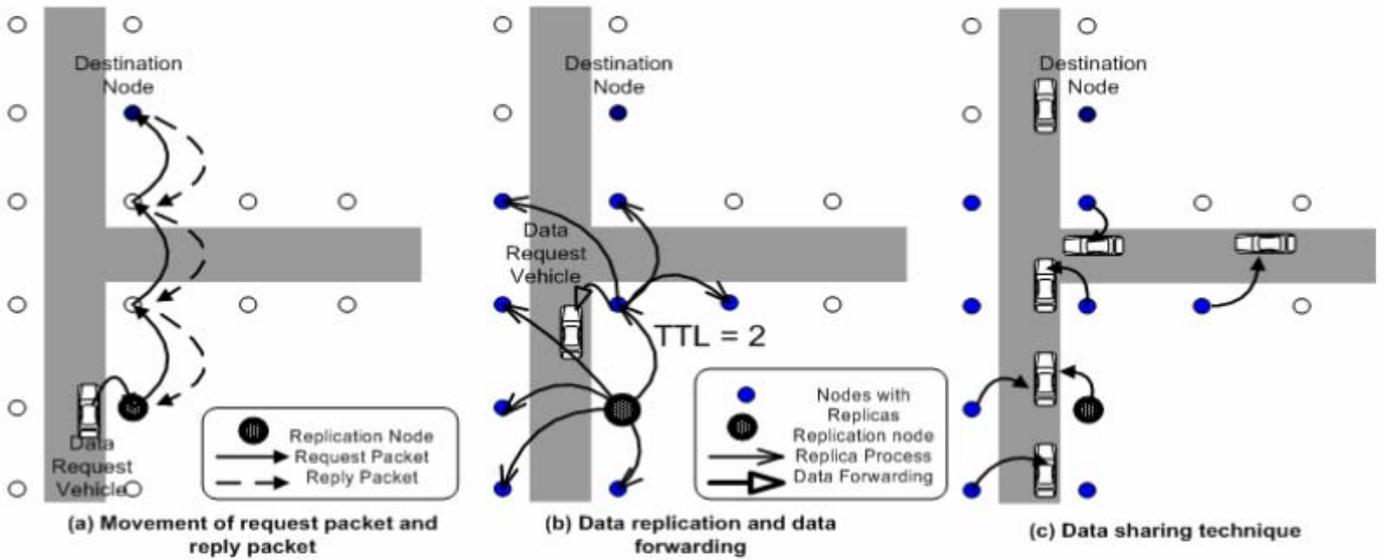
Fig 1. Multi-hop Data Dissemination with Replicas in Vehicular Sensor Networks
