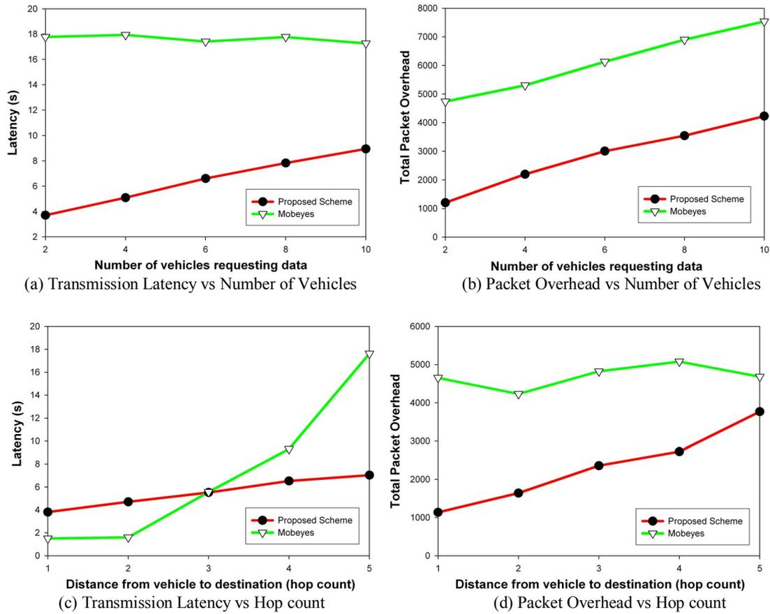
Fig 2. Performance Analysis of the Proposed Scheme in a comparison with Mobeyes [4]
