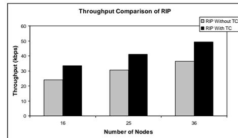
Figure 8. Throughput comparison with RIP routing protocol by applying web-topology formation
