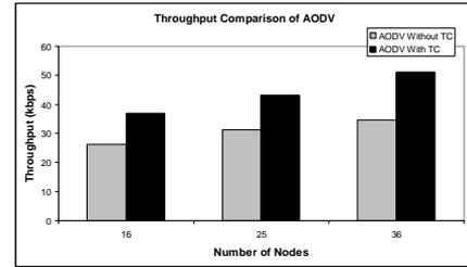
Figure 7. Throughput comparison with AODV routing protocol by applying web-topology scheme
