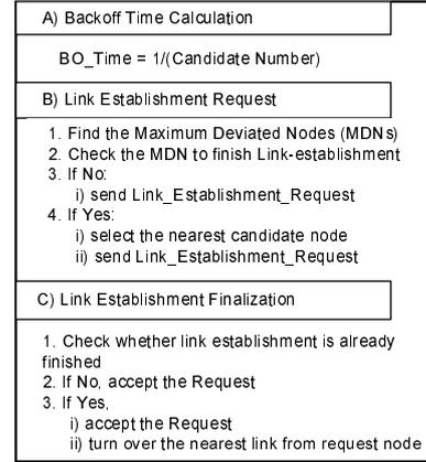
**Figure 2. Two-degree link Establishment Algorithm**
