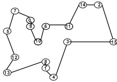
**Figure 4. Link Establishment after phase I in randomly network of 16 nodes**
