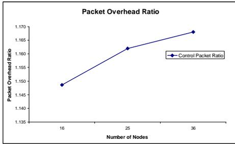
Figure 6. Packet overhead ratio for the topology formation
