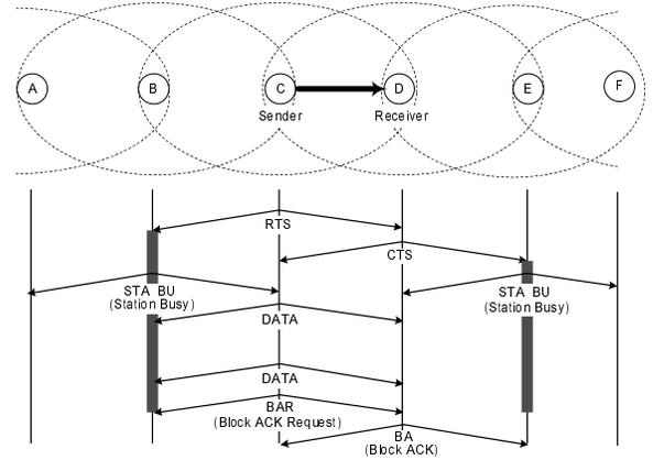
Fig. 2: Aggressive Block ACK Scheme
