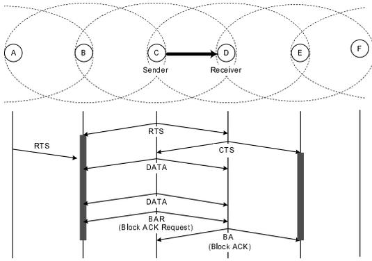
Fig. 1: IEEE 802.11e Block ACK scheme
