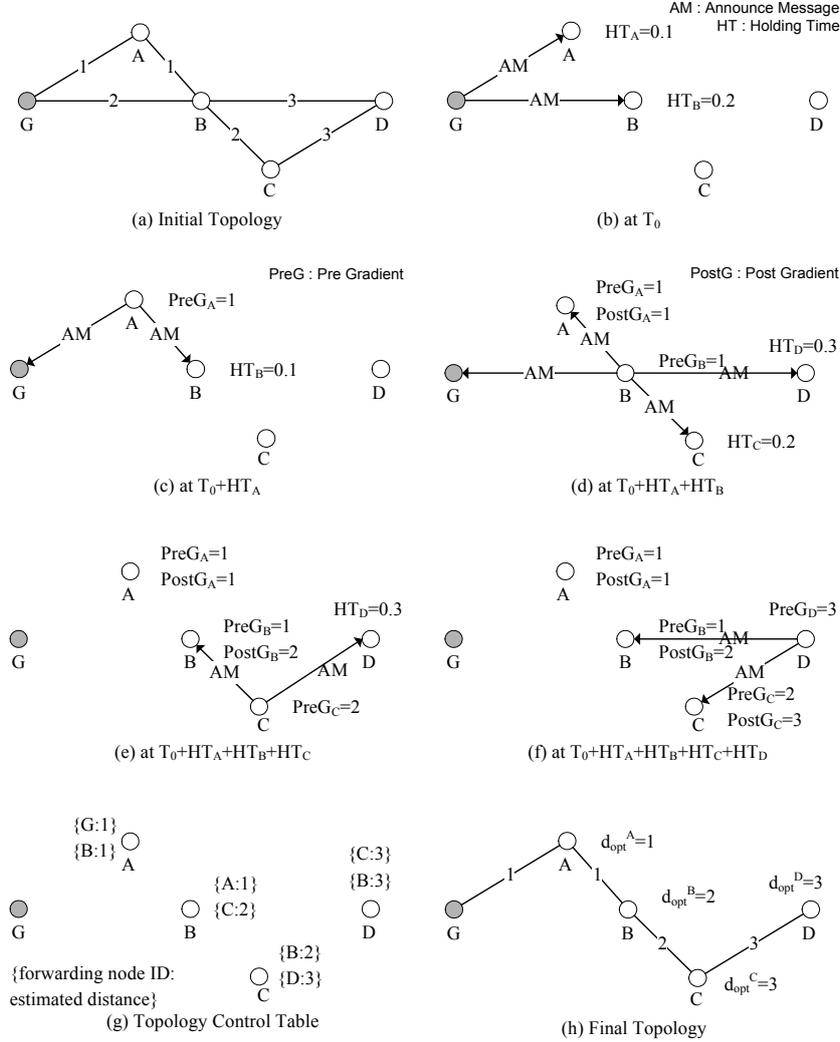
**Fig. 2.** The Sample Flow of DCTC with  $K = 2$
