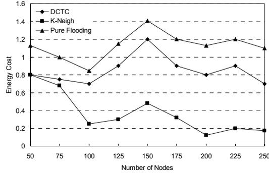
**Fig. 3.** Energy cost of three topology control protocols (DCTC, K-Neigh, and Pure Flooding)
