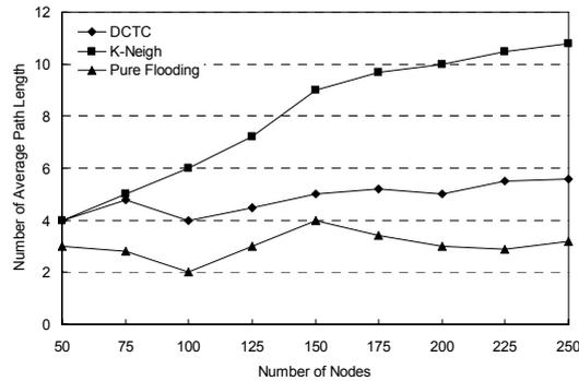
**Fig. 4.** Average path length generated by three topology control protocols
