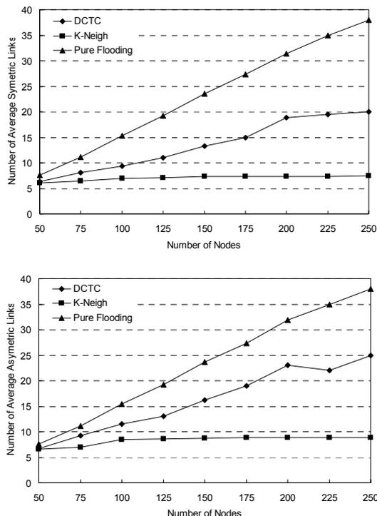
**Fig. 5.** Average logical and physical degree of the topologies generated by the DCTC, K-Neigh, and pure flooding protocols.
