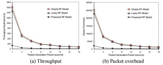
**Fig. 4.** Throughput and packet overhead according to *packet generation period*: number of node is 100, transmission power is -25 dBm and receiver sensitivity is -90 dBm
