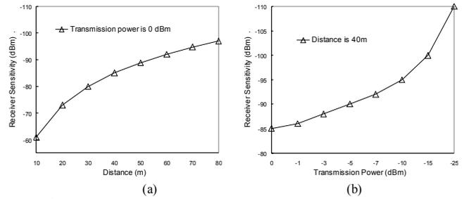
**Fig. 2.** Receiver sensitivity according to the distance and transmission power**TABLE II** SPECIFICATIONS OF THE CC1000[10] AND CC2420[11]
