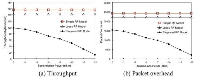
**Fig. 5.** Throughput and packet overhead according to *the transmission power*: the packet generation period is 10 second, number of node is 100 and receiver sensitivity is -90 dBm
