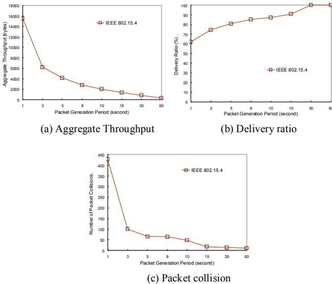
**Fig. 6.** Aggregate throughput, delivery ratio and collision according to the packet generation period: number of node is 10, transmission power is -25 dBm, receiver sensitivity is -90 dBm, SO is 3 and BO is 8
