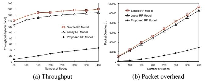
**Fig. 3.** Throughput and packet overhead according to *the number of nodes*: the packet generation period is 10 second, transmission power is -25 dBm and receiver sensitivity is -90 dBm
