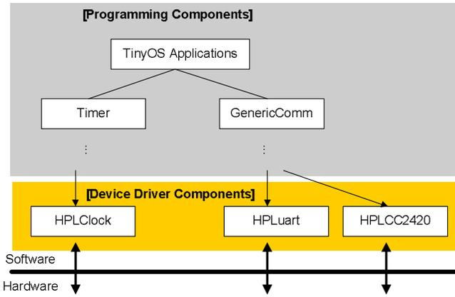
Fig.1. Two component types in the TinyOS
