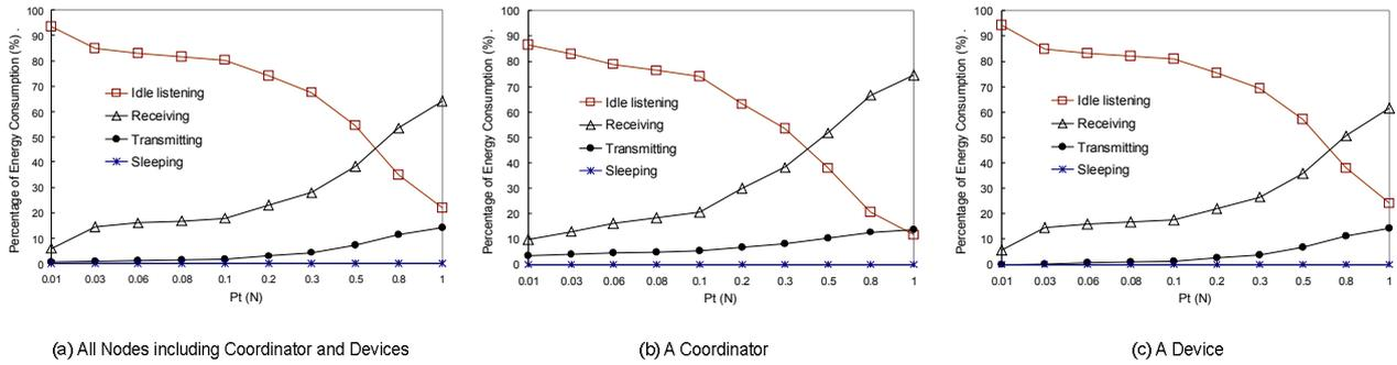
Fig. 4. Percentage of Energy consumptions in four RF states (all nodes, a coordinator and a device)
