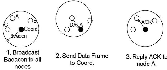
Fig.3. Direct Transmission: Node A tries to transmit its data to coordinator.
