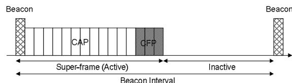
Fig. 1 Super-frame structure in beacon-enable mode [1]
