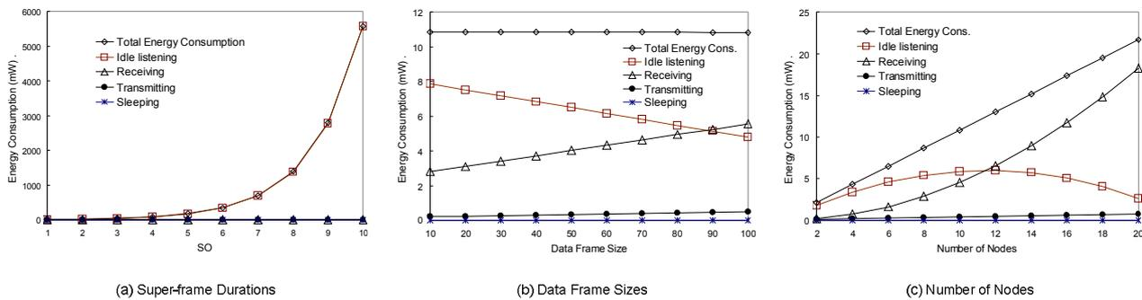
Fig. 5. Energy consumption according to the super-frame duration, data frame sizes and number of nodes
