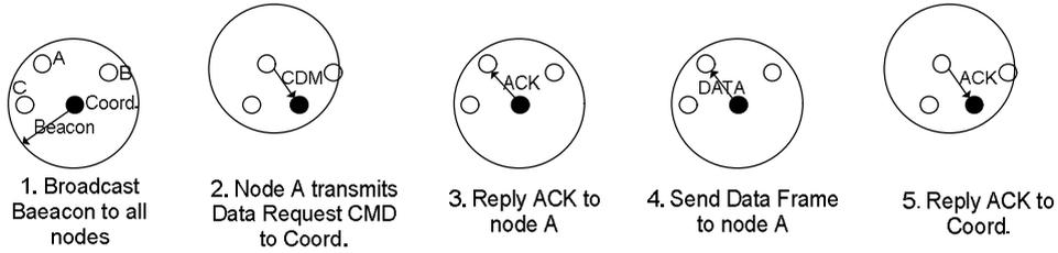
Fig.2. Indirect Transmission: Coordinator tries to transmit its pending data to node A.
