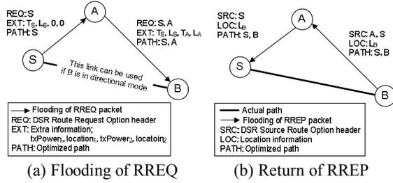
Figure 1. Procedure of our scheme.
