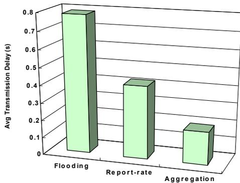
Fig. 6. Average Transmission Delay
