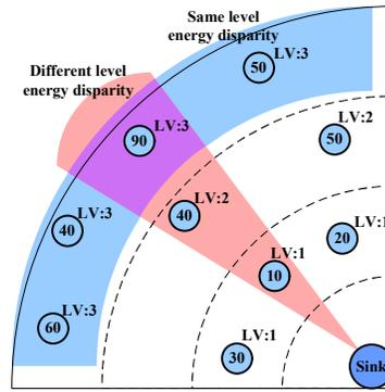
Fig. 1. Two kinds of Energy Disparity in Wireless Sensor Networks (LV : Level, The number in the circle : remained energy)
