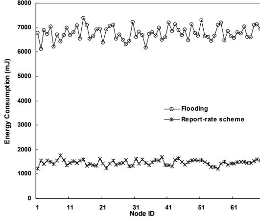
Fig. 4. Energy Consumption in Same Level (level-3)
