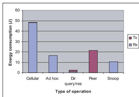
Fig. 3. Energy consumption on various types of operation
